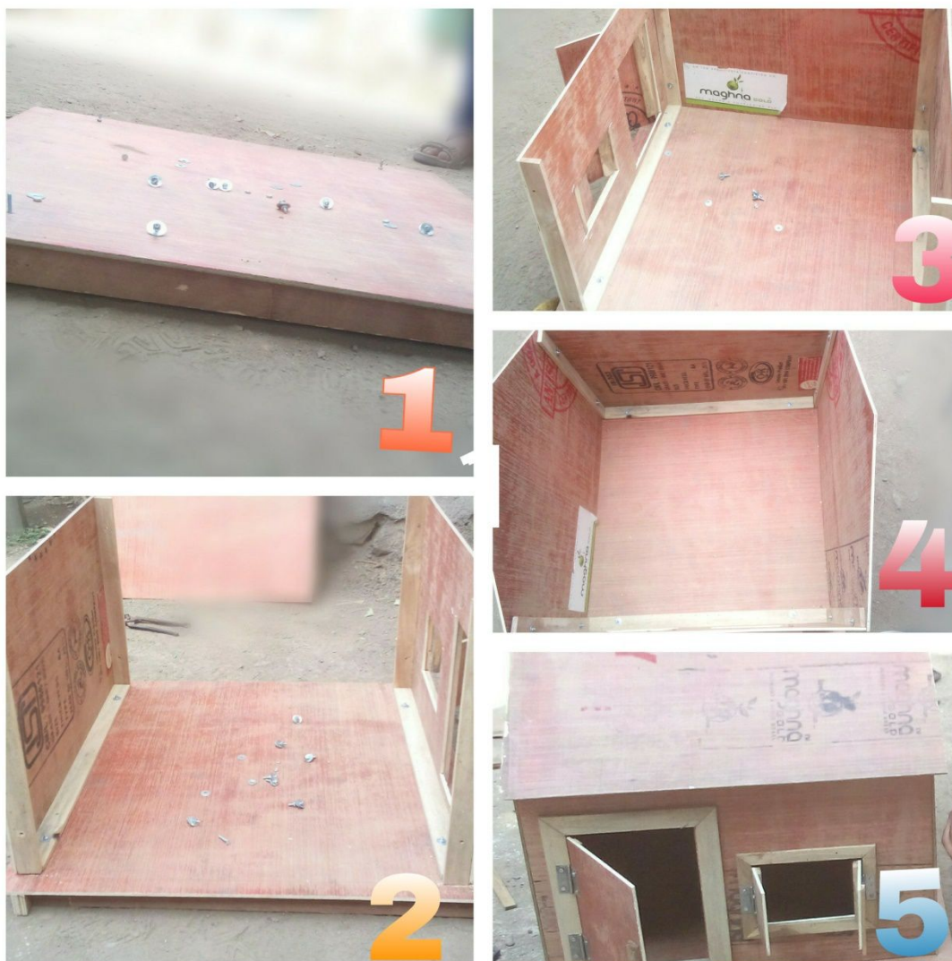
Fig 1. Assembling Of Folding House
